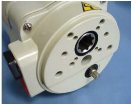
ISO F03/05 Mounting Detail, 8mm socket override and 8 point 14mm female drive on P1 Series actuators.
