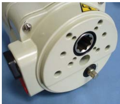
ISO F03/05 Mounting Detail, 8mm socket override and 8 point 14mm female drive on P1 Series actuators.
